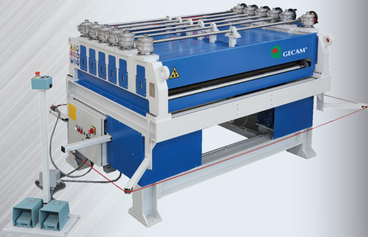
We remove any kind of curvature and undulations of the sheet metal. The levelling are machines that create a plastic deformation process alternating through motorized rollers. Usually are recommended more rollers in case of small thickness and less for thicker sheets metal.
