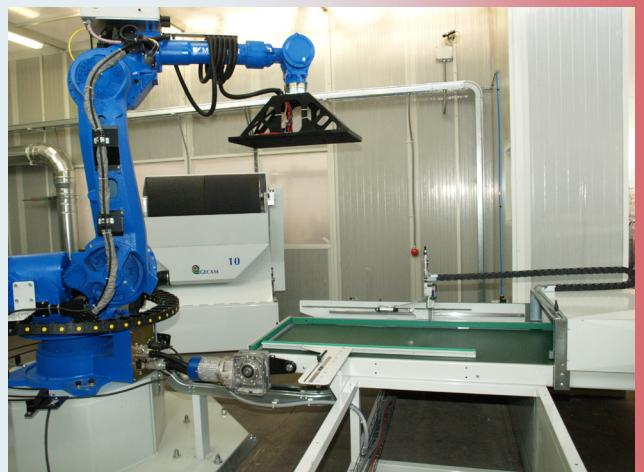
Complete motorized system for grinding and polishing corners and surfaces composed by:
