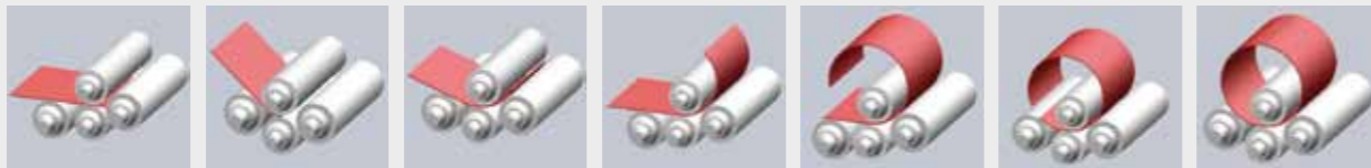
Main phases of 4-roll plate bending. The second pre-bending is obtained without needing to extract and rotate the plate 180°
